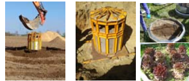
Fig 3: Preparation of the Lysimeter experiments – Fraunhofer IME
